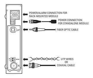
Figure 5. FT8301A Transmitter Connections
